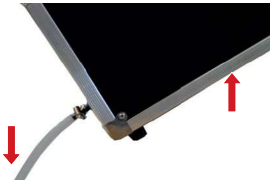
Picture 7-12: Lifting and tilting the pump case
