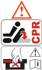
**When the back part is quickly lowered, no foreign object may enter the space between the frame of the bed bearing area, the headboard and the back part. Otherwise it could result in damage or bodily harm!**
