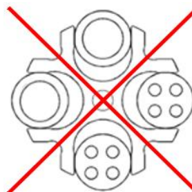
Fig. 9: Permissible and impermissible loading of a swing-out rotor with different tube sizes (example illustration)
