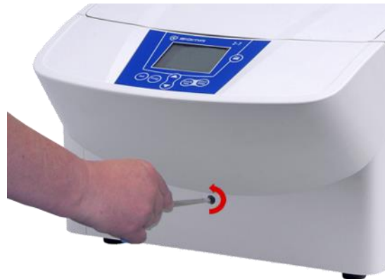
Fig. 15: Manual release of the lid lock
