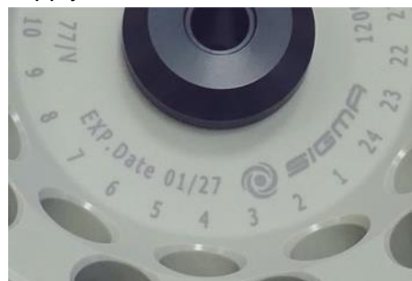
Fig. 5: Different service life – engraving on the bucket/rotor
