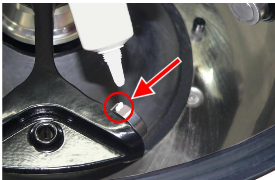
Fig. 16: Sufficient quantity of grease for one bolt
