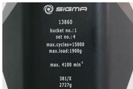
Fig. 4: Different service life – engraving on the bucket/rotor
