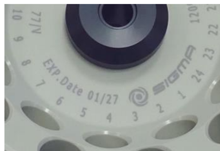
Fig. 4: Different service life – engraving on the bucket/rotor
