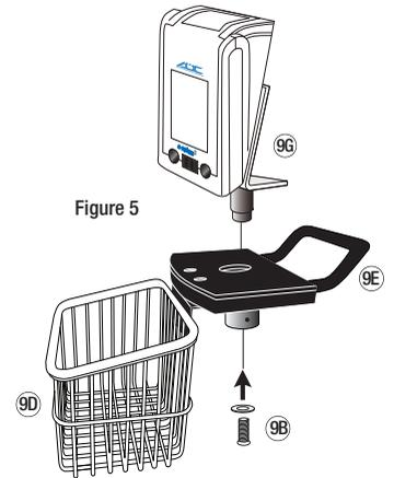
6. Place assembly consisting of the e-sphyg<sup>3</sup>, cuff storage basket and platform on top of stainless steel inner pole, making sure the pole goes completely inside collar. Use tightening device and small hex key as shown. (Figure 6)
