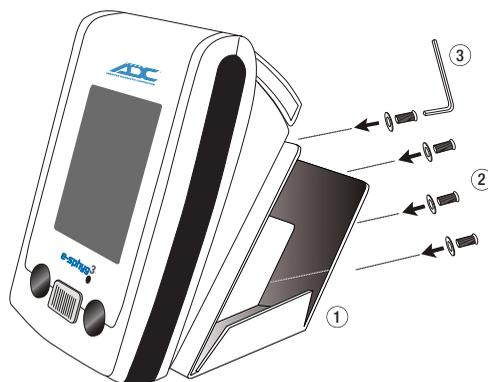
1. Align the holes on the rear side of the e-sphyg<sup>3</sup> with the four holes on the mounting bracket as shown. Insert the four hex mounting screws and washers through the back of the mounting bracket into the unit and tighten. (Figure 1)
